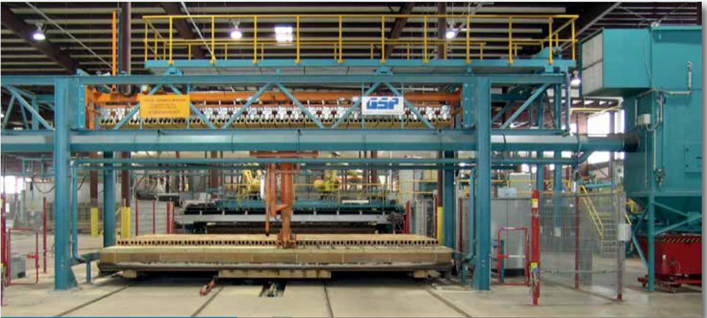
After every firing- and unloading cycle, these kiln car cleaners vacuum the upper deck of the hollow blocks, subsequently lift these blocks and clean the deck underneath as well to prevent the ingress of sand, dust and debris into the core of the kiln cars.
