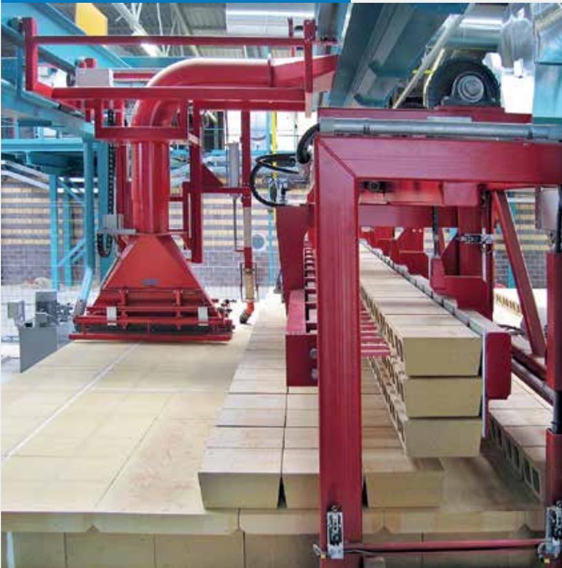
Furthermore the refractories should remain precisely centred on the kiln car deck to enable fault free automatic setting and de-hacking, as well as for stable product transport on the moving cars.
