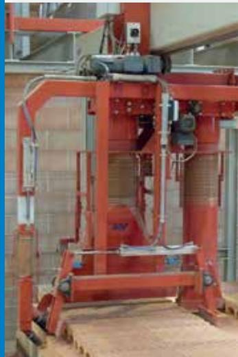
De Boer's Kiln Car Cleaning & Centring Machines range from relatively simple machines, just cleaning the top of the refractories and firing lanes, to machines that raise and re-align all refractories from the kiln car deck, whilst cleaning the bare kiln car deck underneath.
